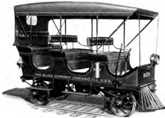
Buda No. 100. Inspection Motor Car, Nine Passengers
